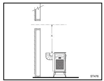
Fig. 26 Determine the vertical pipe length.
